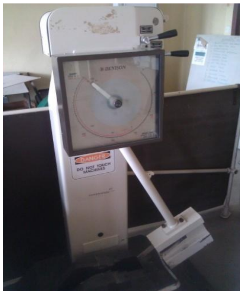
Figure 3.8: Photograph of Avery Denison impact tester.
