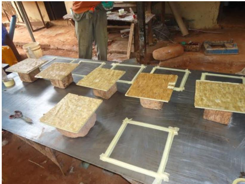
Fig. 3.1: Mould set-up for fiber-reinforced composites, CCRD, Nsukka
