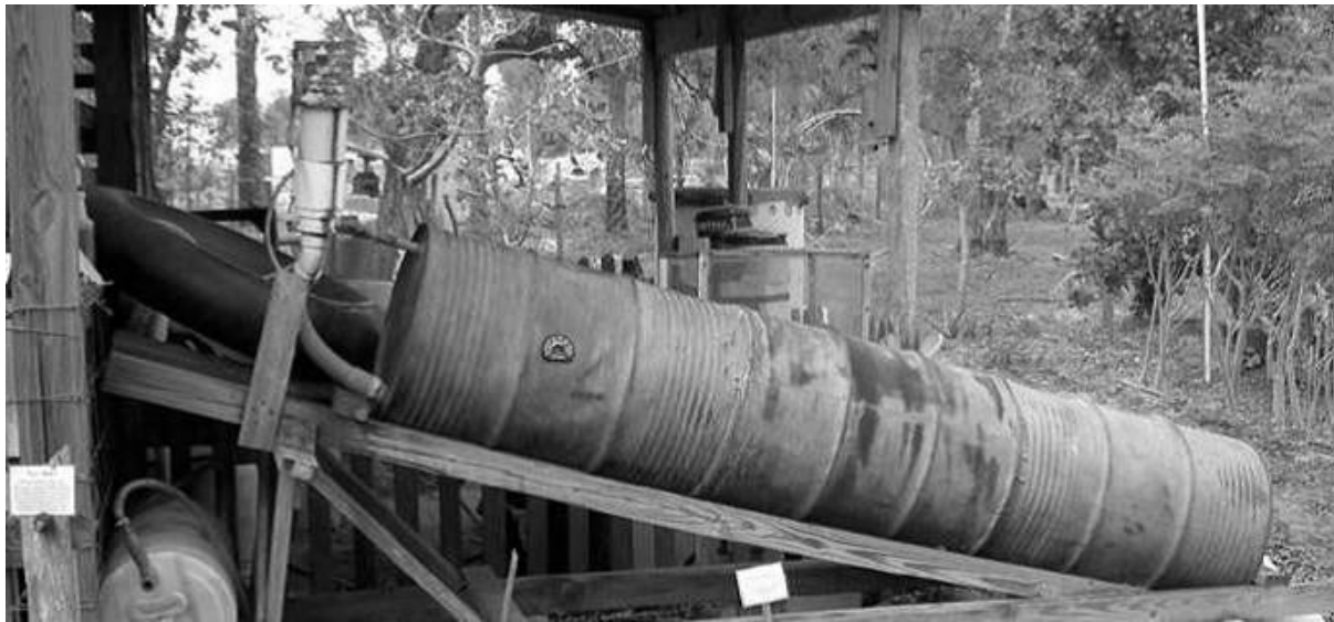
Fig. 2.15: A flow-thru digester (Source: Doerr and Lehmkuhl, 2008)
