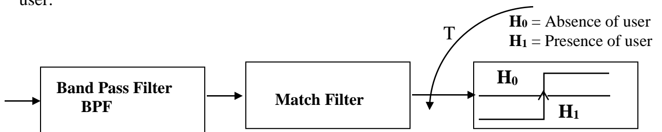
Figure 3.4: Diagram of matched Filter detection Model (Garhwal and Bhattacharya (2011))
