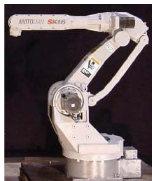
Figure 2.4: The parallelogram revolute manipulator (Spong et al, 2006)
