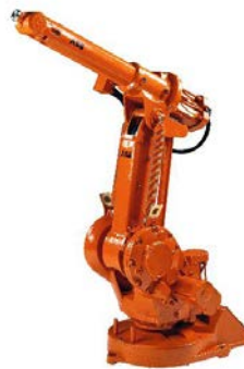
Figure 2.3: The articulated revolute manipulator (Spong et al, 2006)
