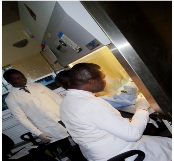
Figure 4.27: Samples Preparation in Biosafety Cabinet CLASS II for Real Time PCR
