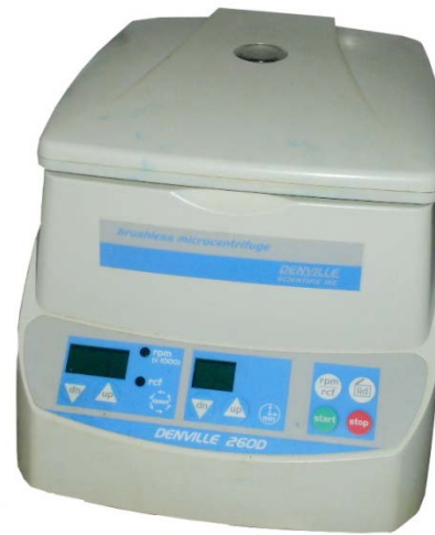
Figure 4.25: Denville 260D Microcentrifuge used for DNA Extraction for Conventional PCR
