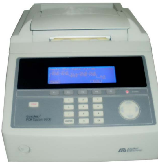
Figure 4.28: GeneAmp PCR System 9700 Thermal cycler used for Conventional PCR
