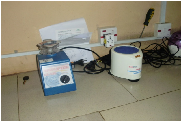
Figure 4.24: Vortex Machines for Mixing of Samples and Reagents before Centrifugation
