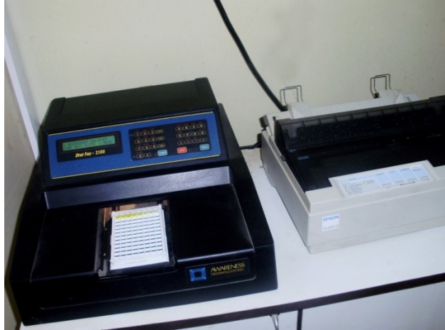
Figure 4.22: Stat fax 2100 Plate Reader and Printer used for all ELISA Procedures
