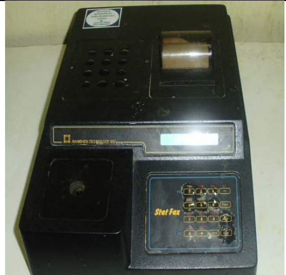
Figure 4.23: Stat Fax 1904 Spectrophotometer Used for Determination of Alanine Aminotransferase (ALT)
