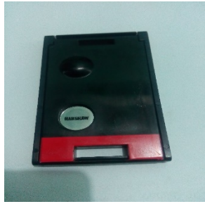
Figure 2.6: Thermoluminescent dosimeter chip in a casing.
