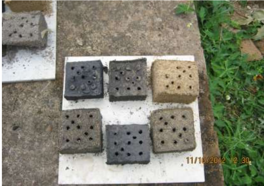
Plate 5: Samples of coal-rice husk briquettes made using \text{CaSO}_4 as binder.
