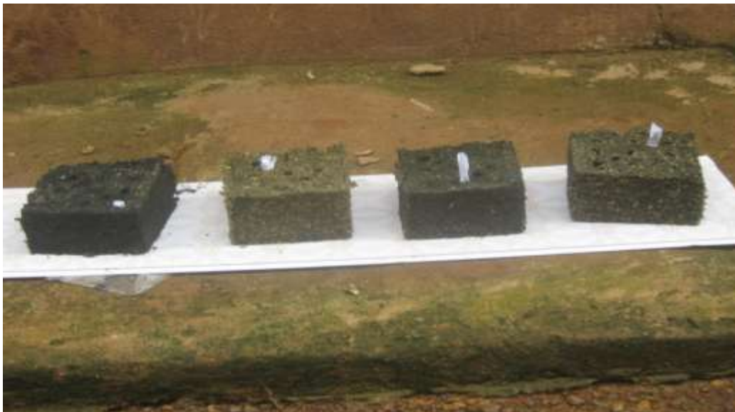
Plate 8: Sample of coal-corn cob briquettes produced with cement as binder.
