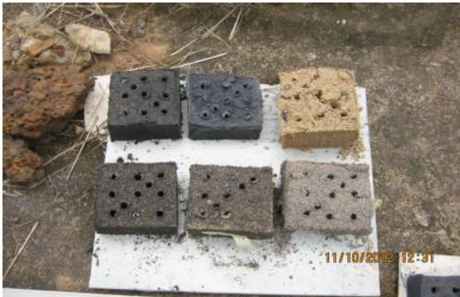
Plate 6: Samples of coal-rice husk briquettes made using starch as binder.
