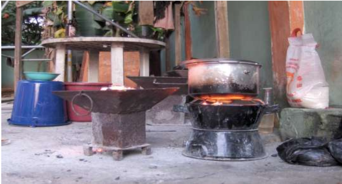
Plate7: A typical coal briquette stove used for cooking in Ikwo, Ebonyi state. Ash is collected in a compartment below the briquettes, making it easier to clean.
