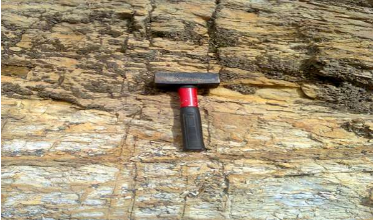
Plate 4.6: Fractures in Outcrop of the Olive Brown shale observed at Hausa quarters
