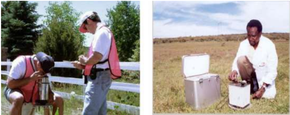
Fig. 2.3: The Worden and LaCoste - Romberg gravity meters (Mariita, 2007)
