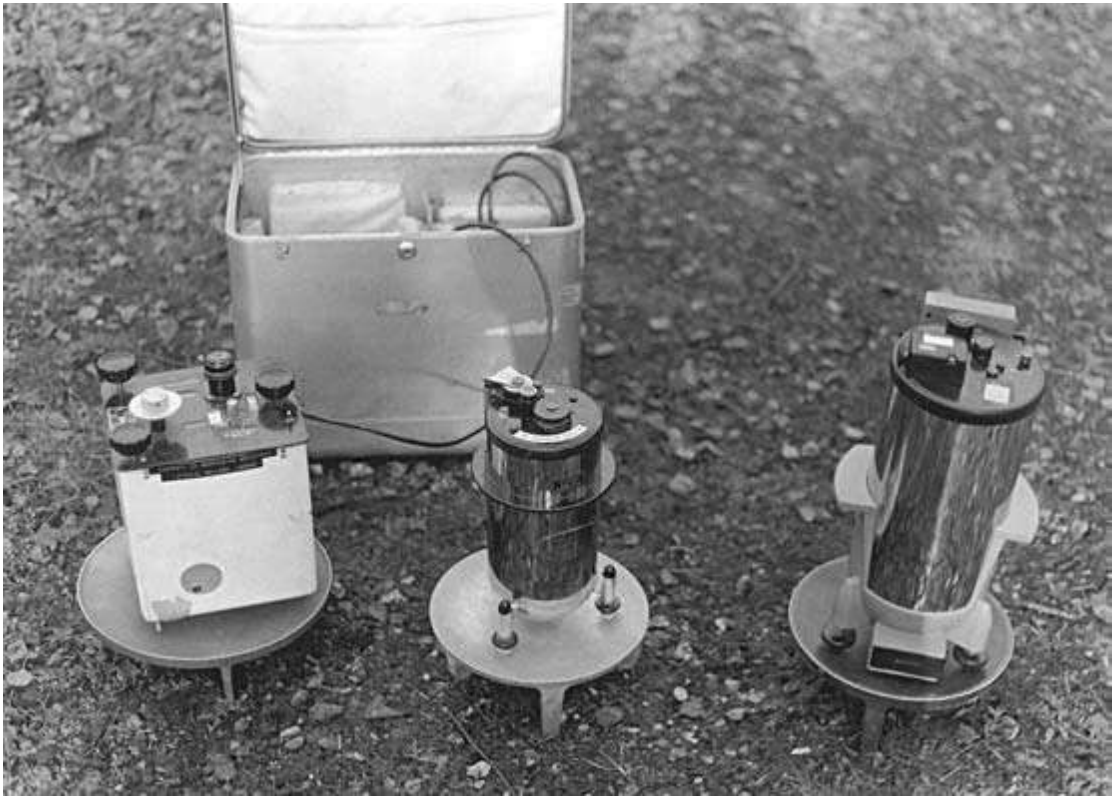
Fig. 2.4: ‘Manual’ gravity meters. From left to right, LaCoste ‘G’ (geodetic), Worden ‘Student’ and Sodin. (After Milsom, 2003)
