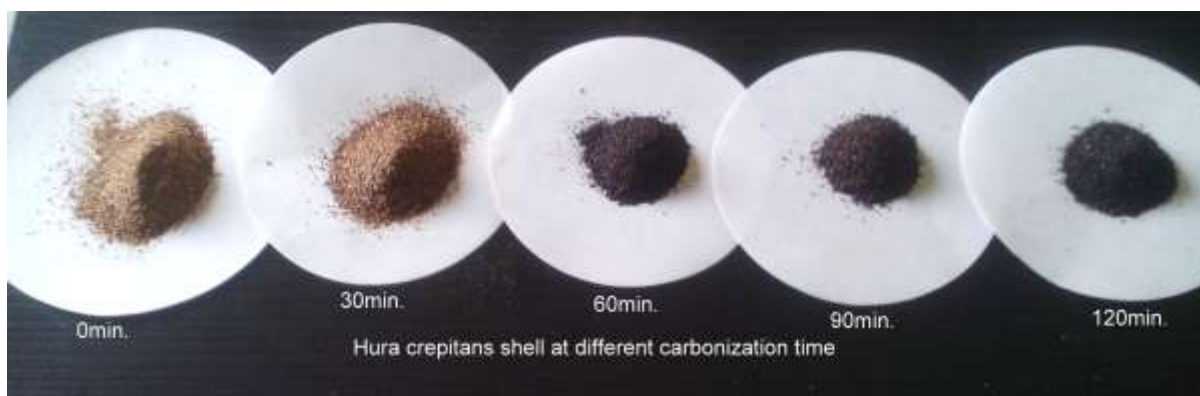
Plate 3.6: H. crepitans Seed shell carbonized at 500 °C at Varied Time
