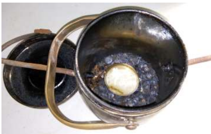
Plate 3.8: Locally constructed carbonizer
