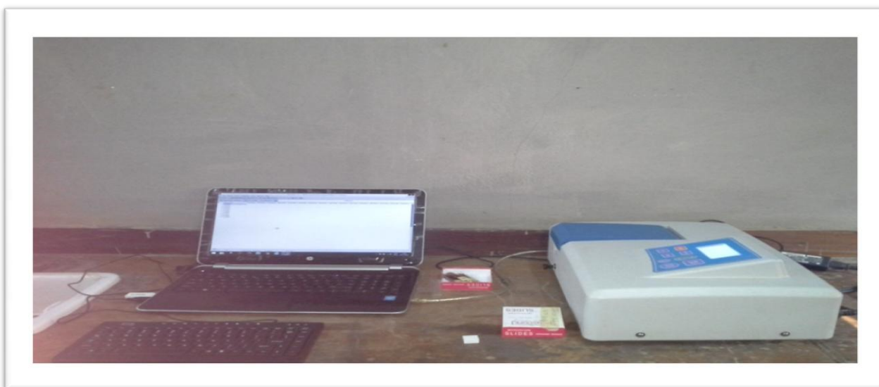
Plate 3.9: Ultraviolet Visible MetaSpecAE1405031Pro Spectrophotometer, Wavelength range: 200-1000nm.
