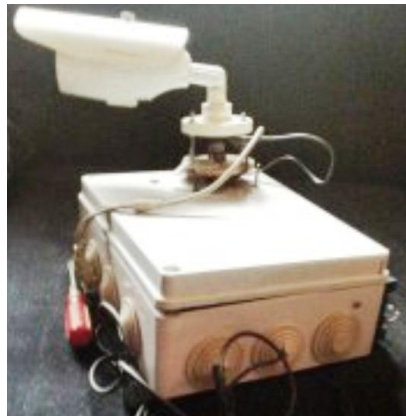
Figure 3.22: Client station with surveillance camera
