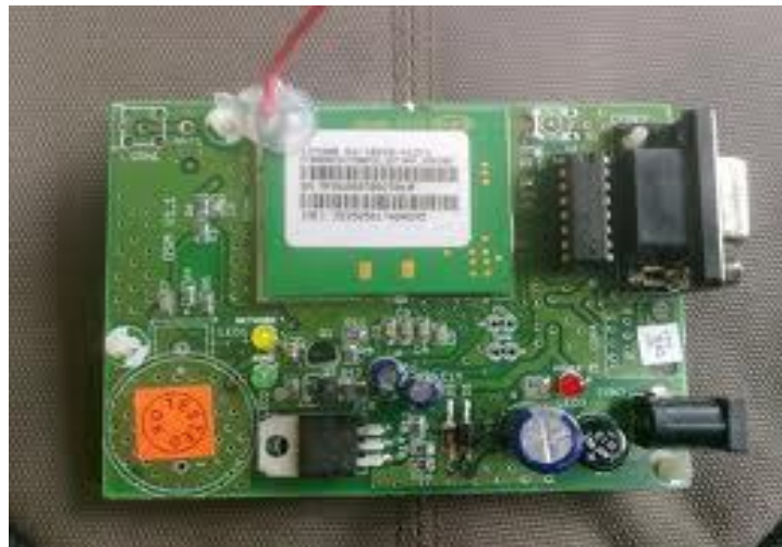
Figure 3.11: Snapshot of SIM 300S GSM Tx/Rx Module
