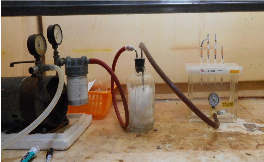
Plate 3.4: The smoking regime and entrapment of TSNAs by the prepared MIP samples.
