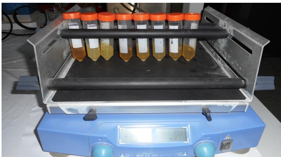
Plate 3.6: Rotatory shaker with the secured eluted materials from the MIP SPE.
