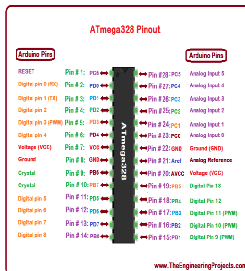
Figure 3.16: The Pin-out of ATmega328P microcontroller (Nasir, 2017)
