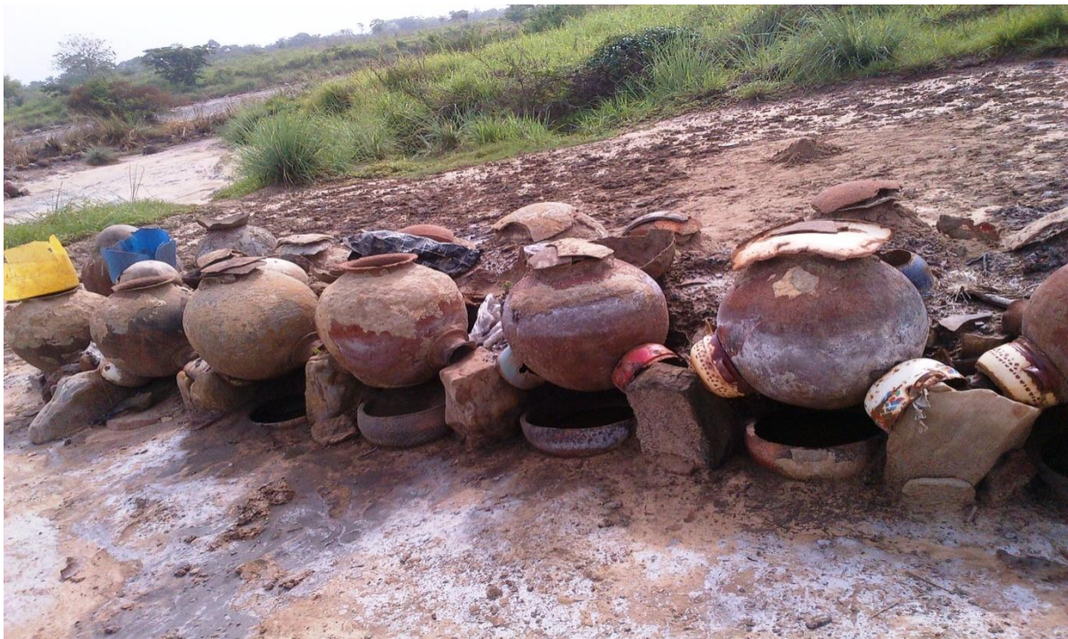
Photo i: First stage of the producton process. Filtration pots filled with the salt water at the lake.
