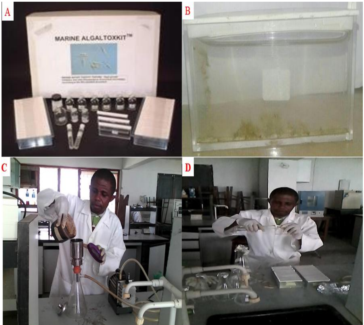
Appendix IIe: Features of the marine toxicity test with microalga A. Contents of the Algaltoxkit.
