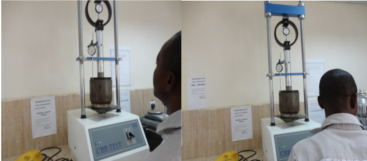
Plate 20: Showing the loading of sample by C.B.R machine for top and bottom respectively
