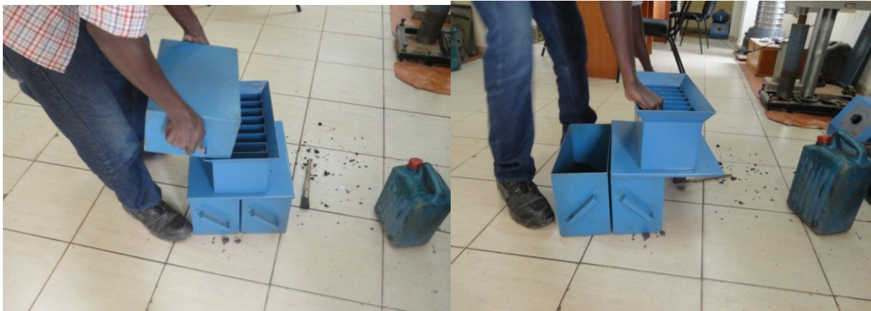
Plate 8; shows quartering of sample using Raffle Box
