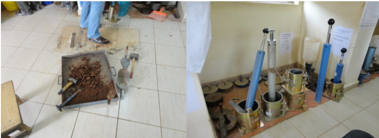
Plate 18 and 19: Showing tray and 4.5 & 2.5kg rammer used to mix sample thoroughly.
