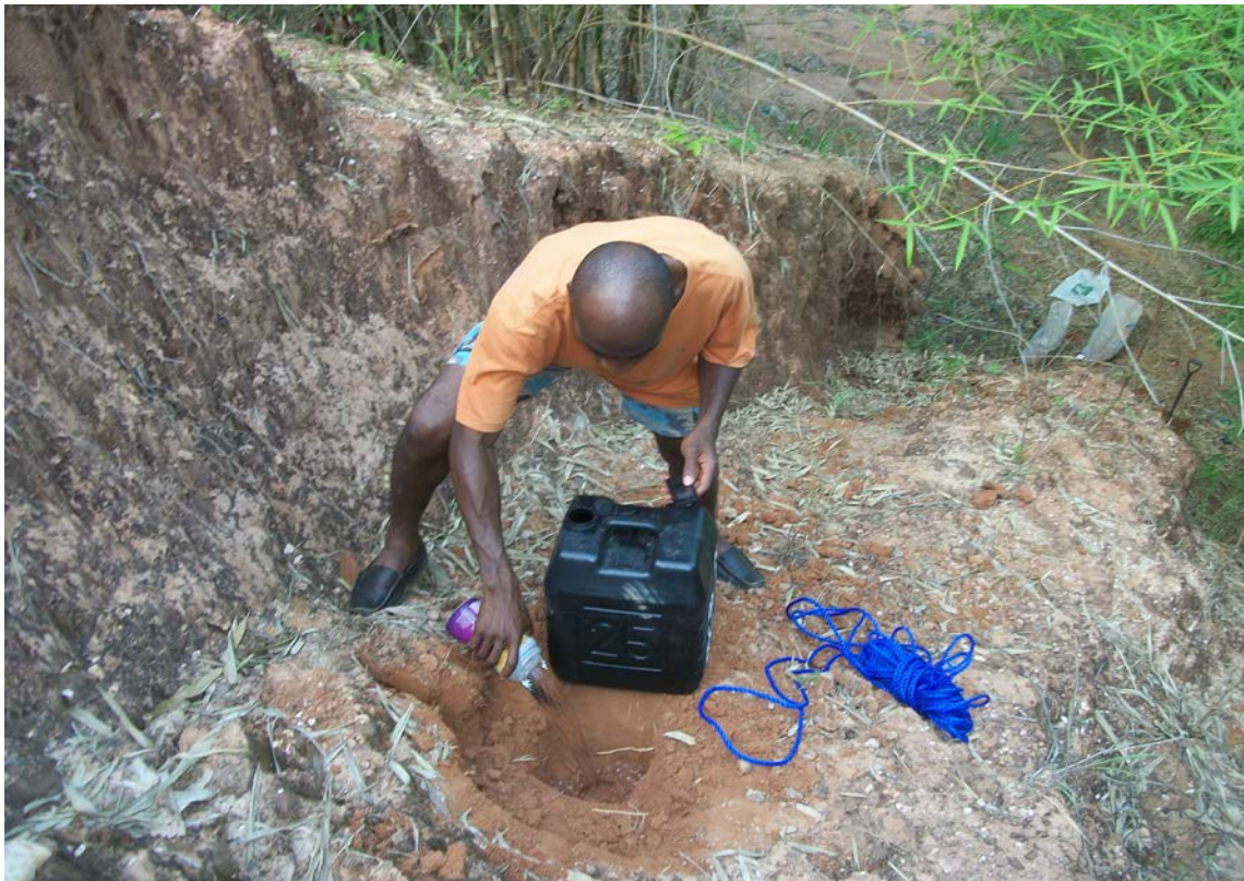
Plate 7; Percolation test being carried out at B-Horizon in Agulu Erosion site (Photoshot, Emeka, 2012)
