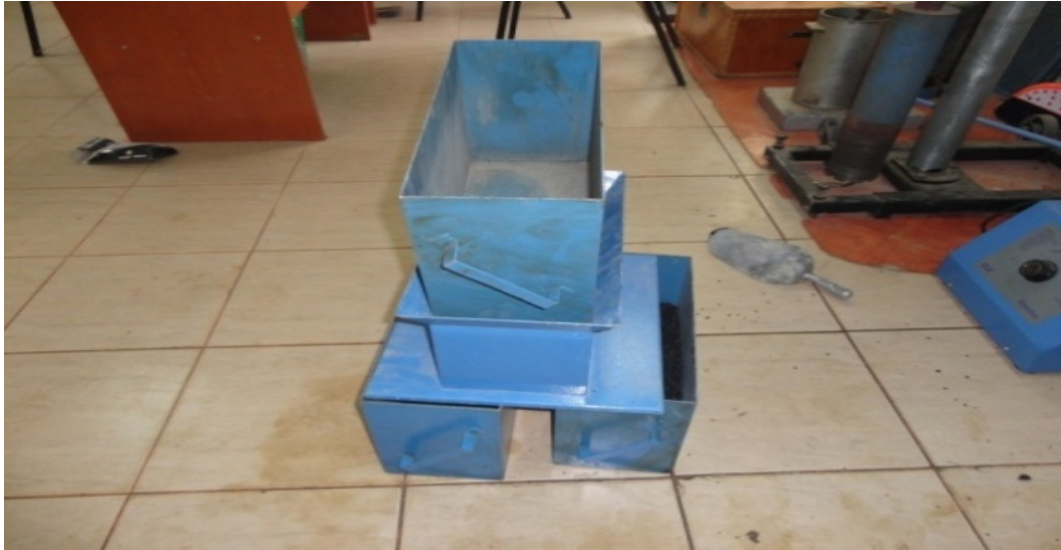
Plate 17 showing raffle box used to quarter sample.
