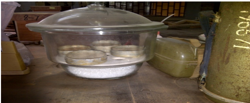
Plate 12 shows specimens for specific gravity in the desiccators.
