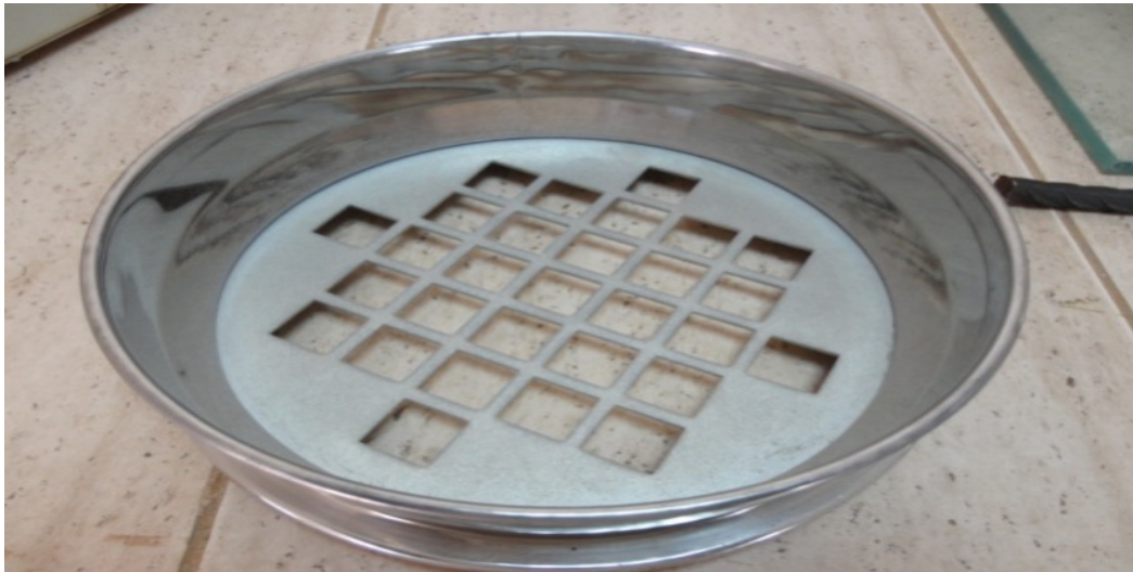
Plate 16 showing 19mm sieve used to sieve sample.
