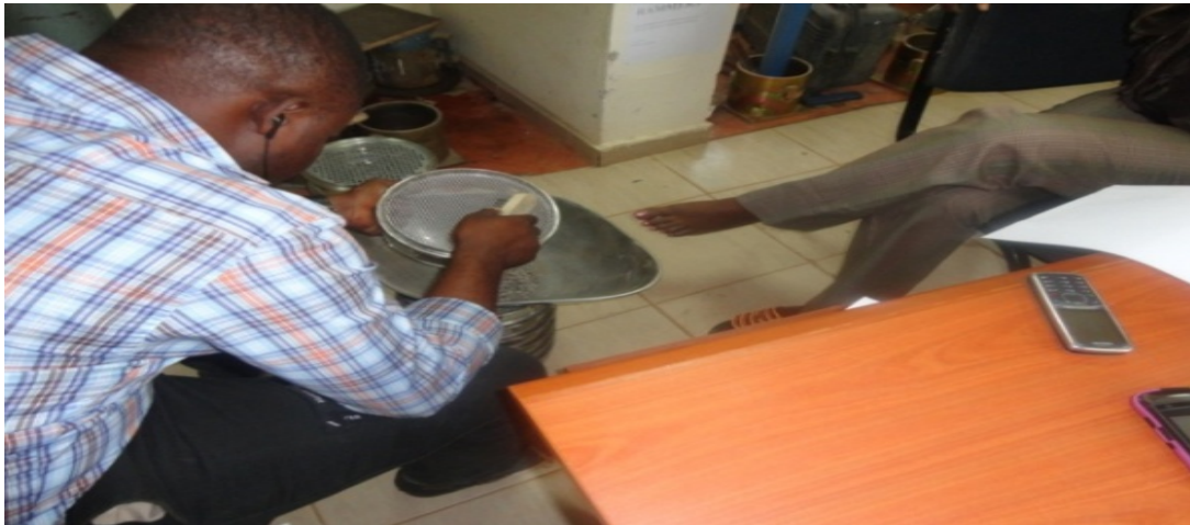
Plate 11: showing wire brushing of sieve to remove all particles
