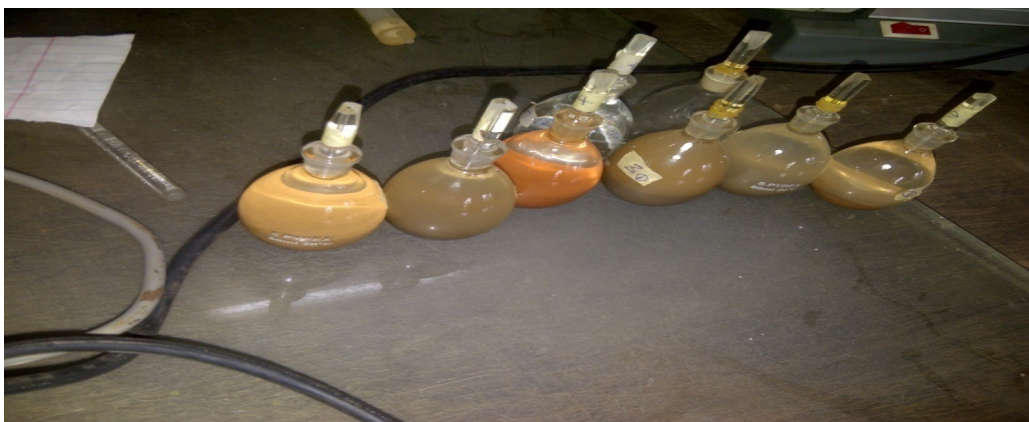
Plate 13 shows pycnometer + sample + water, thus observe that the sample is covered by water
