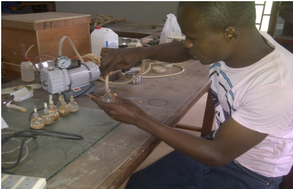
Plate 14 shows removal of air bobbles gently using the vacuum pump assisted by Nonso Okeke, Lab. Technologist.
