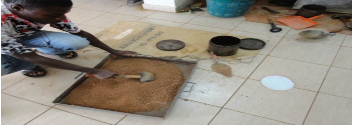
Plate 15 showing dislodging of sample using rubber hammer
