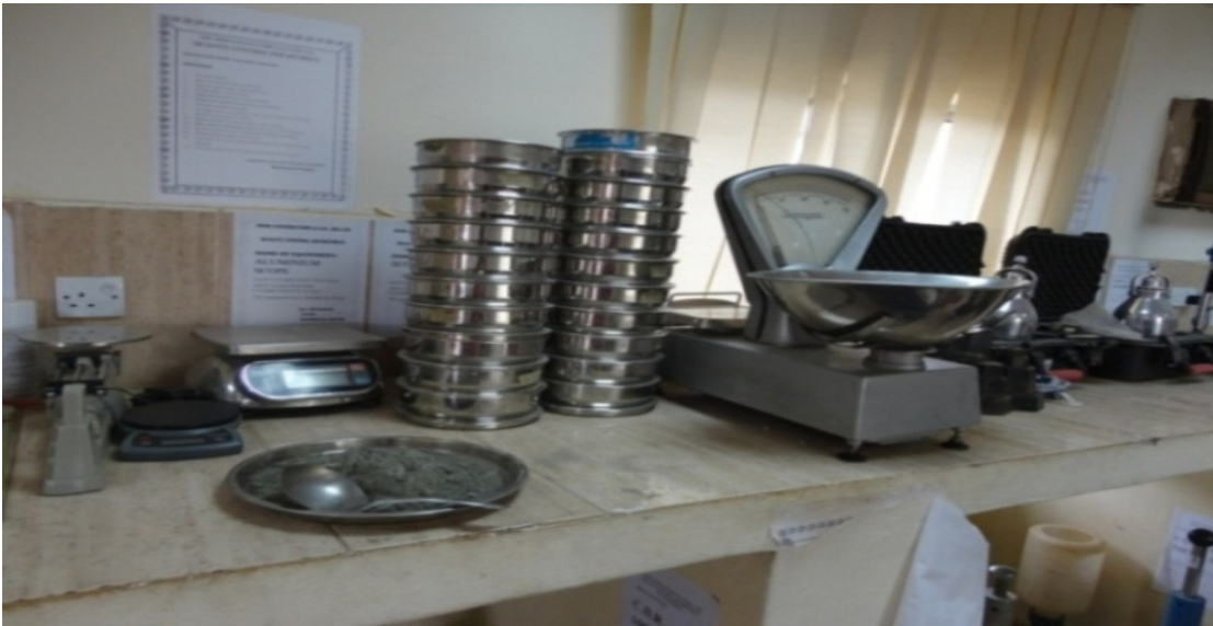
Plate 9 showing the arrangement of sieves according to diameter of aperture
