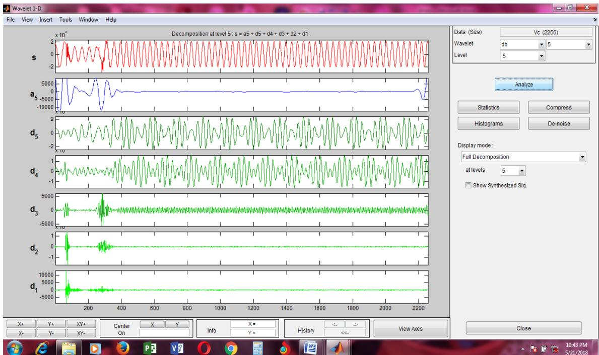
P21: Decomposed signal of voltage waveform of LLL Fault of phase C at a distance of 140km from the source
