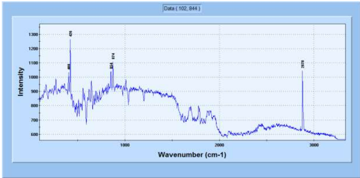
Figure 4.1 Raman spectrum of ZnO nanoparticles produced with SLS.
