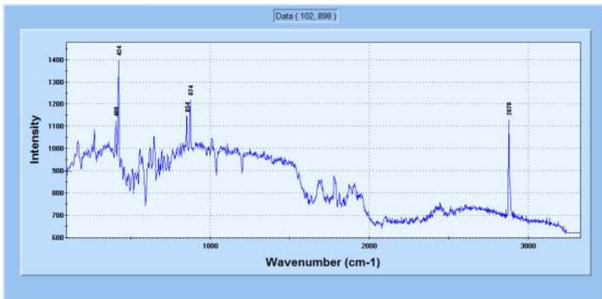
Figure 4.2 Raman spectrum of ZnO nanoparticles produced with LABS.
