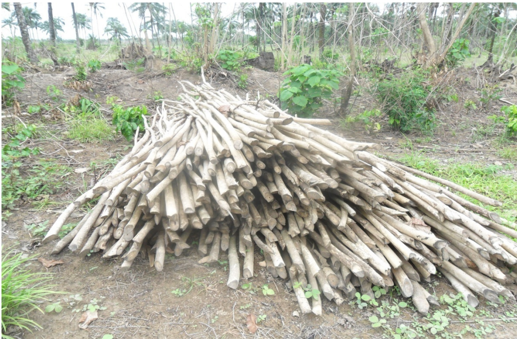
Plate 10: premature woods of tectona grandis cut for scaffolding by the natives
