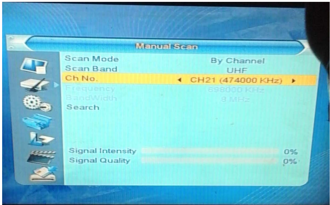
Figure 3.10. A DVB-T2 decoder showing DVB-T2 channels. It shows that channel 21 with 474000 KHz frequency is unoccupied in that particular zone. Also figure 3.11, shows that channel 50 with frequency 706,000 KHz is occupied in that zone, the signal intensity is 72% while the signal quality is 97%.
