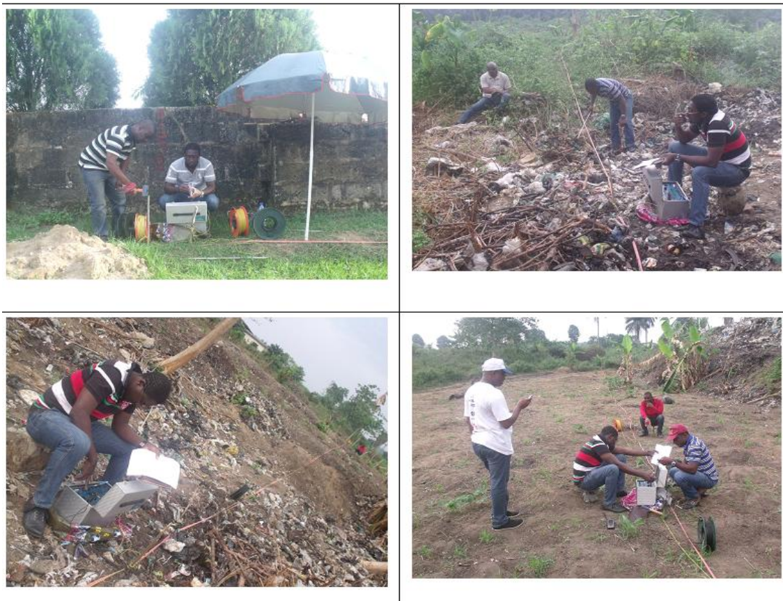
Fig. 3.4: Field procedures and data acquisition during Resistivity Survey.
