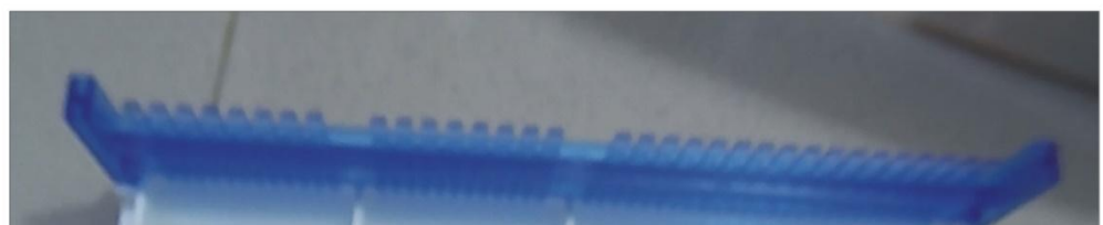
Plate 11: (o) Gel electrophoretic cast with appropriately fixed gel comb and leveler, (p) Eppendorf's tubes containing extracted HBV and HCV DNA samples, (q) Gel electrophoretic cast with appropriately fixed gel comb and agarose gelin Prof Tاتفeng Mirabaue Molecular Laboratory Niger Delta University, Bavela.
