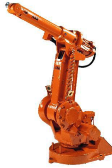
Figure 2.3: The articulated revolute manipulator (Spong et al, 2006)
