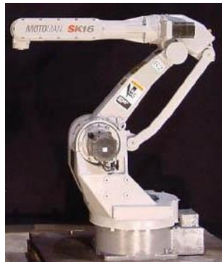
Figure 2.4: The parallel revolute manipulator (Spong et al, 2006)
