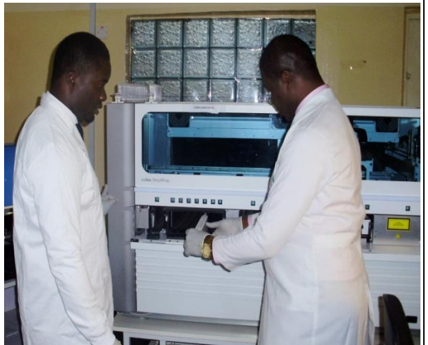
Figure 4.29: Loading of Samples in COBAS AmpliPrep for Nucleic Acid extraction for Real Time PCR
