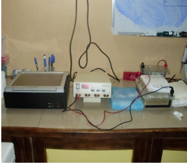
Figure 4.30: UVP Trans illuminator for Gel Visualization and tank for Agarose Gel Electrophoresis
