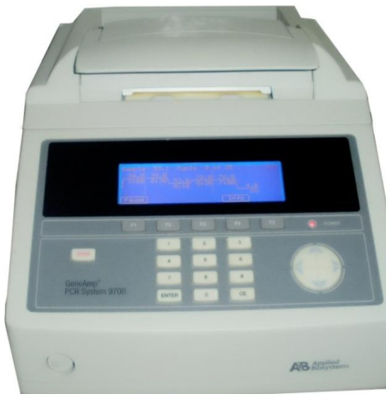
Figure 4.28: GeneAmp PCR System 9700 Thermal cycler used for Conventional PCR
