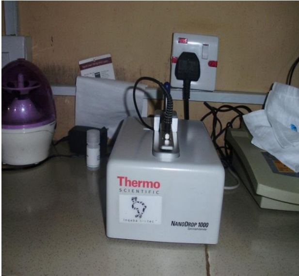
Figure 4.26: Thermo Scientific NanoDrop 1000 Spectrophotometer Used for Detection and Assessing the Quality of DNA after Extraction
