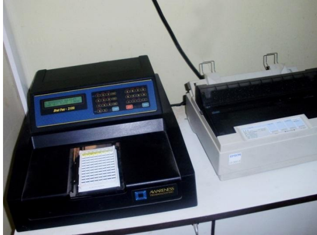
Figure 4.22: Stax fax 2100 Plate Reader and Printer used for all ELISA Procedures
