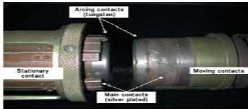
Figure 2.12: Tulip Contacts in Dell-Alsthom air-blast Circuit Breaker (Nasrallah et al, 2007).
