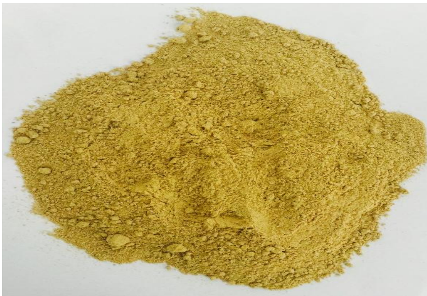
Figure 3.6 Powdered ginger rhizomes with Thermal Conductivity of 0.0503W/m.K
