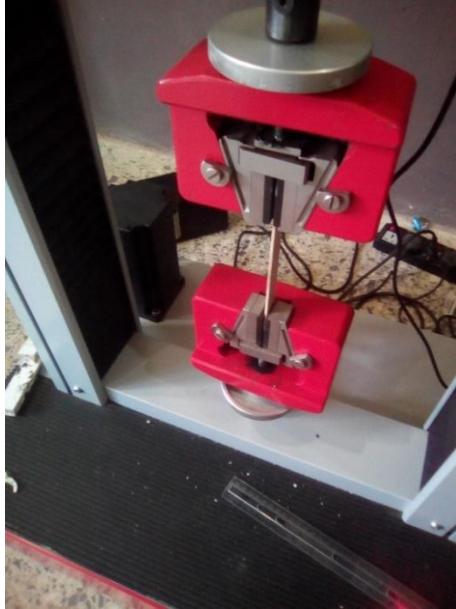
Plate 3.2: Substrate bond pair mounted on a tensile machine
