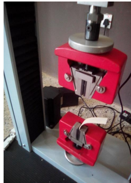
Plate 3.3: Substrate bond pair break on a tensile machine
