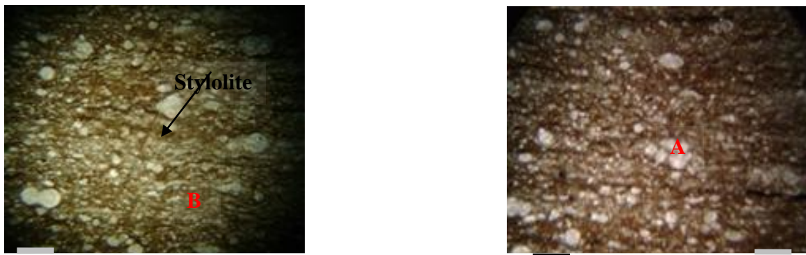
Figure 4.48: Photomicrograph of OT.5.3 showing (A) Planktic foraminiferal tests (B) Micrite (microcrystalline calcite and kaolinite) Bar scale = 2 mm Magnification: \times 50 Resolution:
