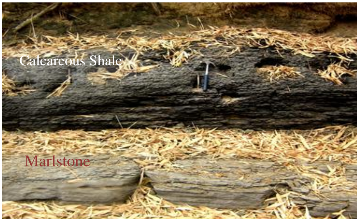
Figure 4.9: Marl and Shale unit showing good fissility
