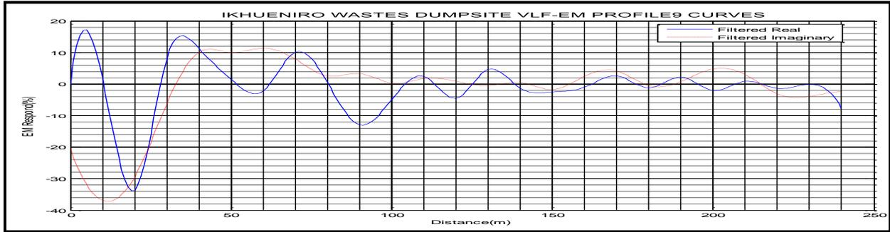
**Fig. 4.13a: Ikhueniro VLF-EM Curve (filtered real and filtered imaginary) of Profile (PL9)**
