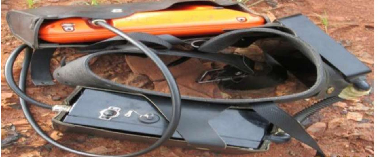
Fig. 3.8: ABEM Wadi and Accessories used for the VLF Electromagnetic Survey
