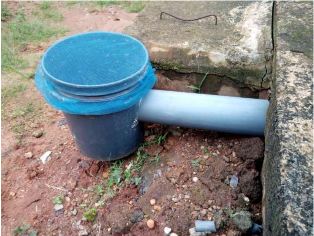
Locally made emergence trap used in collecting emerging adult mosquitoes from Septic tanks
