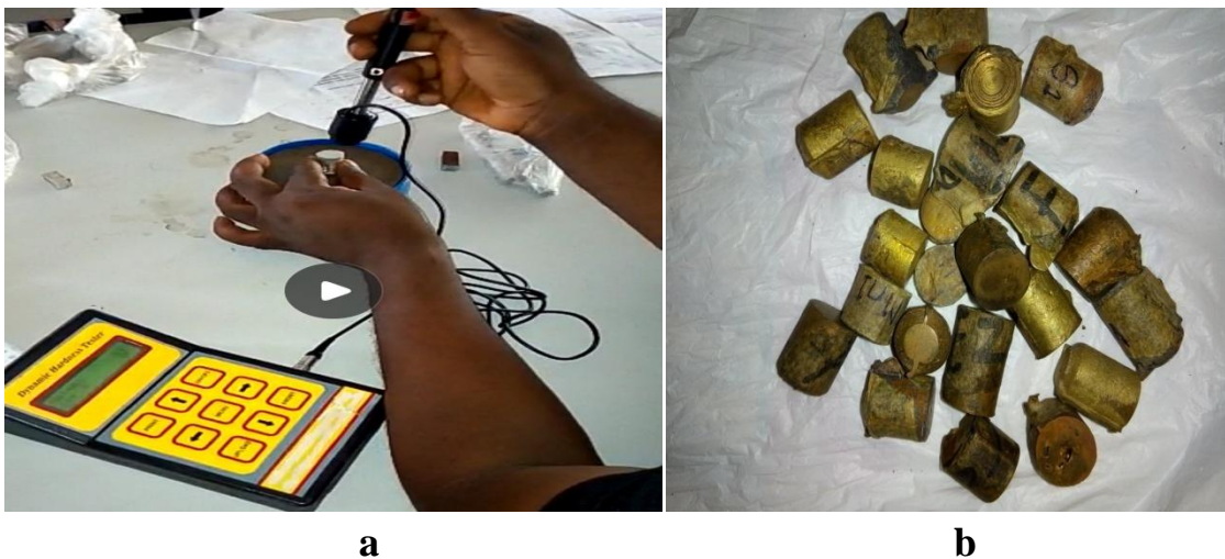
Figure 3.6: (a) Brinell hardness test procedures and (b) Tested samples
