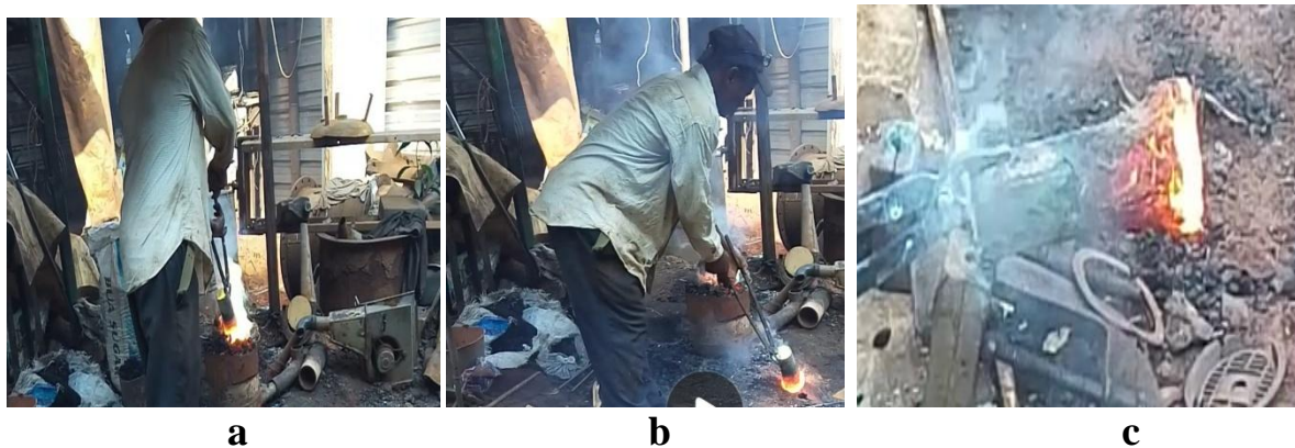
Figure 3.3: (a) Melting of materials, (b and c) Casting of samples
