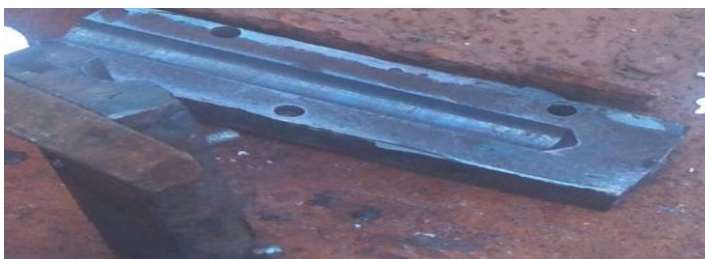
Figure 3.1: Mould for casting
