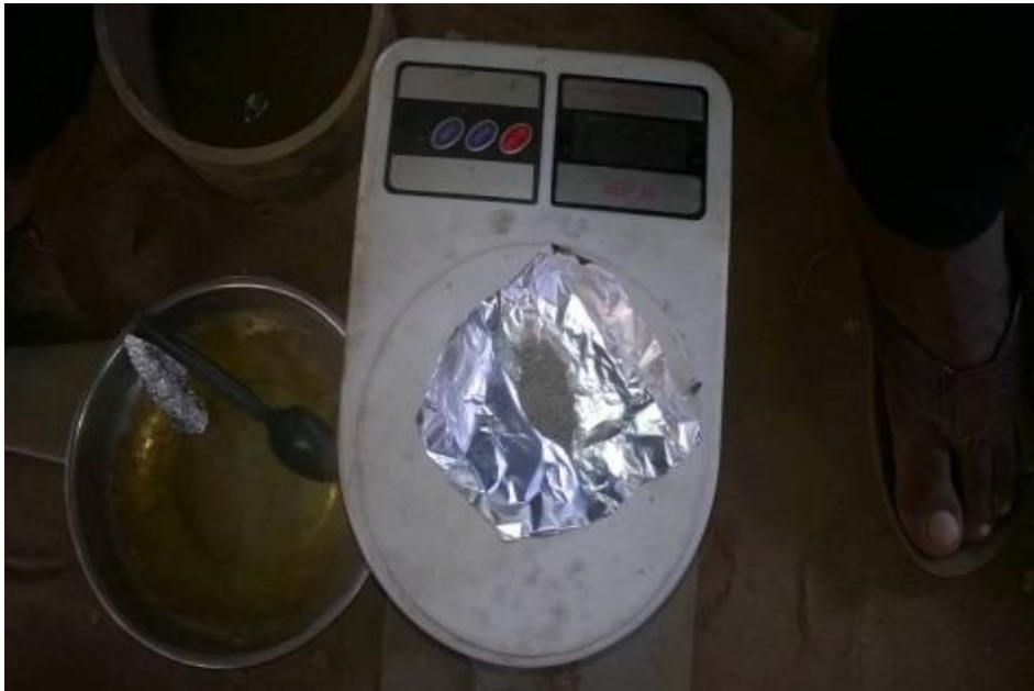
Figure (d) represents the process of measuring out carbide forming elements using electronic weighing balance.
