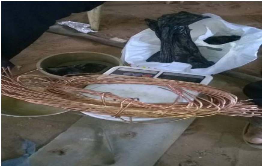
Figure (b) represents the process of measuring out copper using electronic weighing balance.
