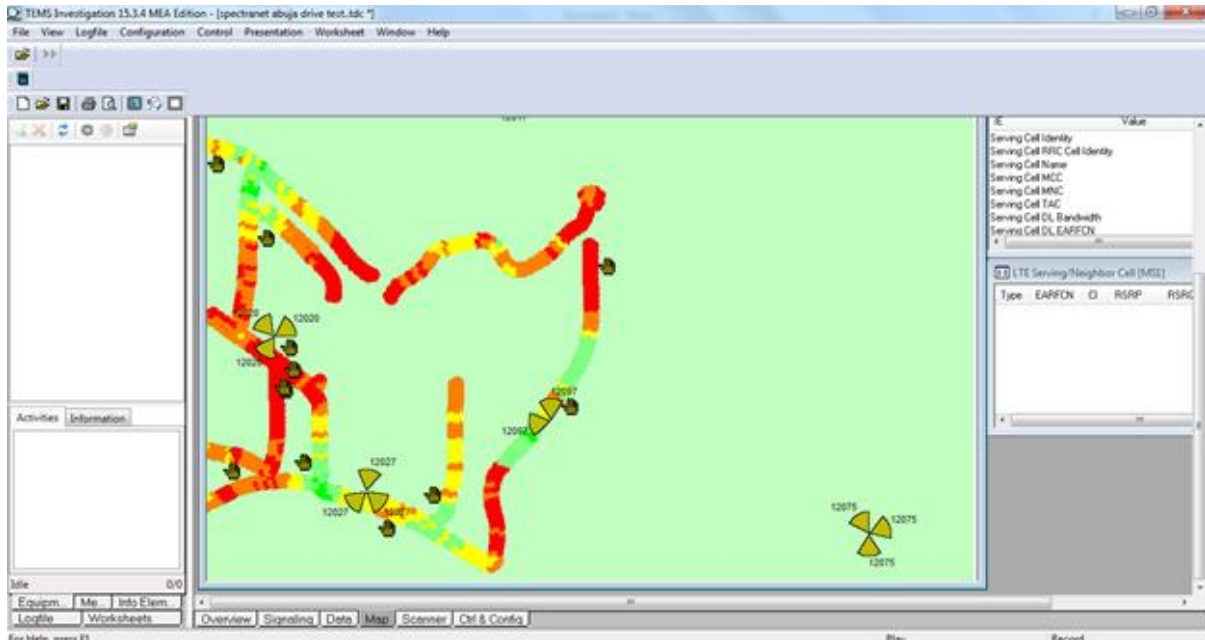
Figure 4.36: Drive Test for Optimization over GVARIMPA eNodeB Sites
